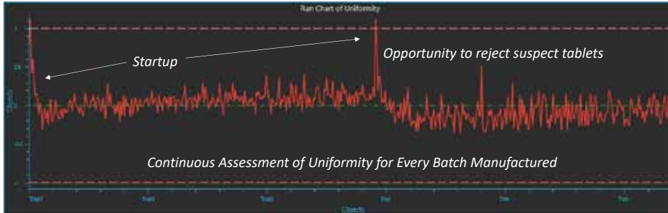
Figure 5: Control chart of a tablet compression run monitored by NIR spectroscopy.
